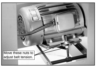
Figure 32. Adjusting belt tension.
